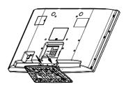
Finally secure the bottom-plate with 2 screws (supplied).
